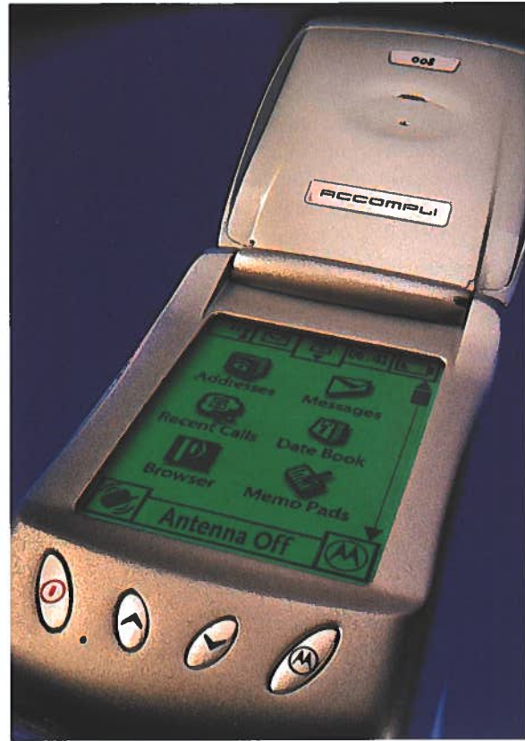
▲ Photo 1 Gadget? GPRS terminal and dual band GSM mobile phone from Motorola with handwriting and speech recognition.
